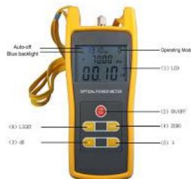
Gambar 5. Optical Power Meter (OPM)
